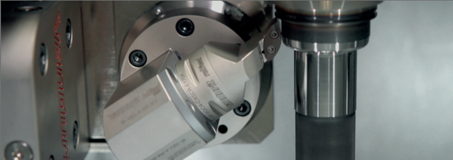
Kugelgelenk (Hartdrehen) Feinschlichten + drall-frei | ball joint (hard part turning) fine-finishing + twist-free
